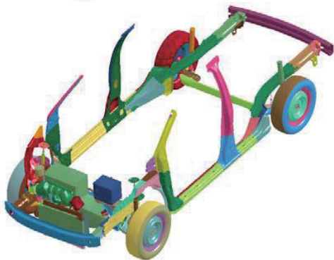
Fig. 2 – Details of the Modeled Vehicle Frame and Drive Train
