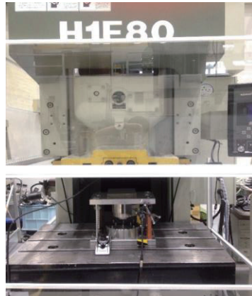
Fig.2 800kN Mechanical Link Servo Press
